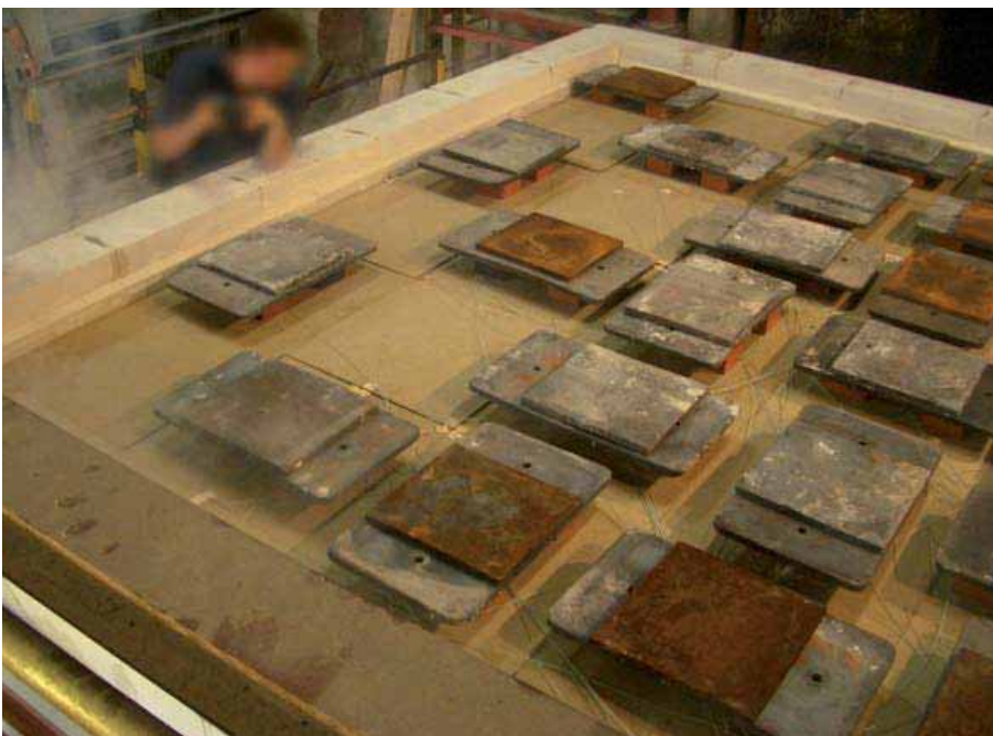
Fire resistance performance test of a system floor under load according to DIN 4102/2.
